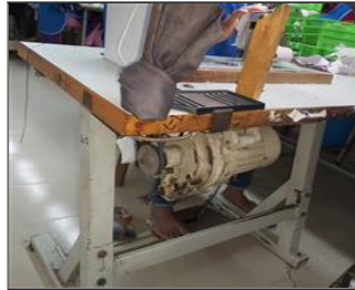
Photo of non-conformity Pully cover found missing.JPG
