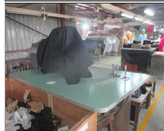
Photo of non-conformity Band knife machine found without safety barrier.JPG
